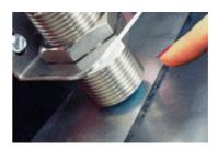
The contribution to the process is detection equipment that inspects the shell for doubles at the infeed and verify that the tab is present at the discharge of the machine. Logically these are two different applications. The first is a typical double detector and the latter is a missing part detector, even though we utilize identical metal thickness detection circuits.
